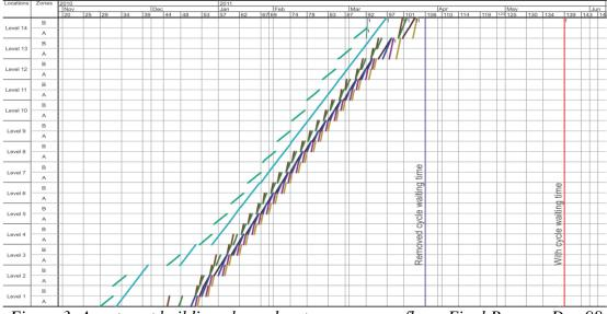
Figure 3: Apartment building planned as two pours per floor. Final Pour on Day 98
