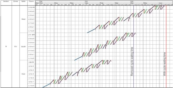
Figure 4: Educational building in three wings with the structural cycle organised as a single run per floor. Total duration 185 days, Wing 3 duration 107 days
