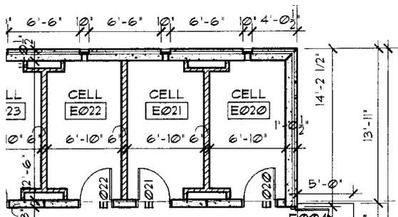
Figure 2: Plan View of Prison Cells
