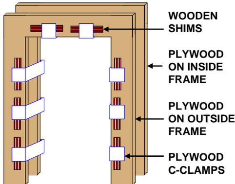
Figure 10: Diagram of Plywood Fix
