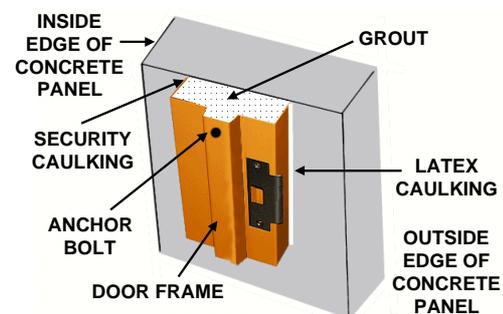
Figure 3: 3-D Diagram of Frame Design
