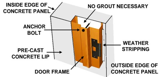
Figure 11: Concrete Lip Fix
