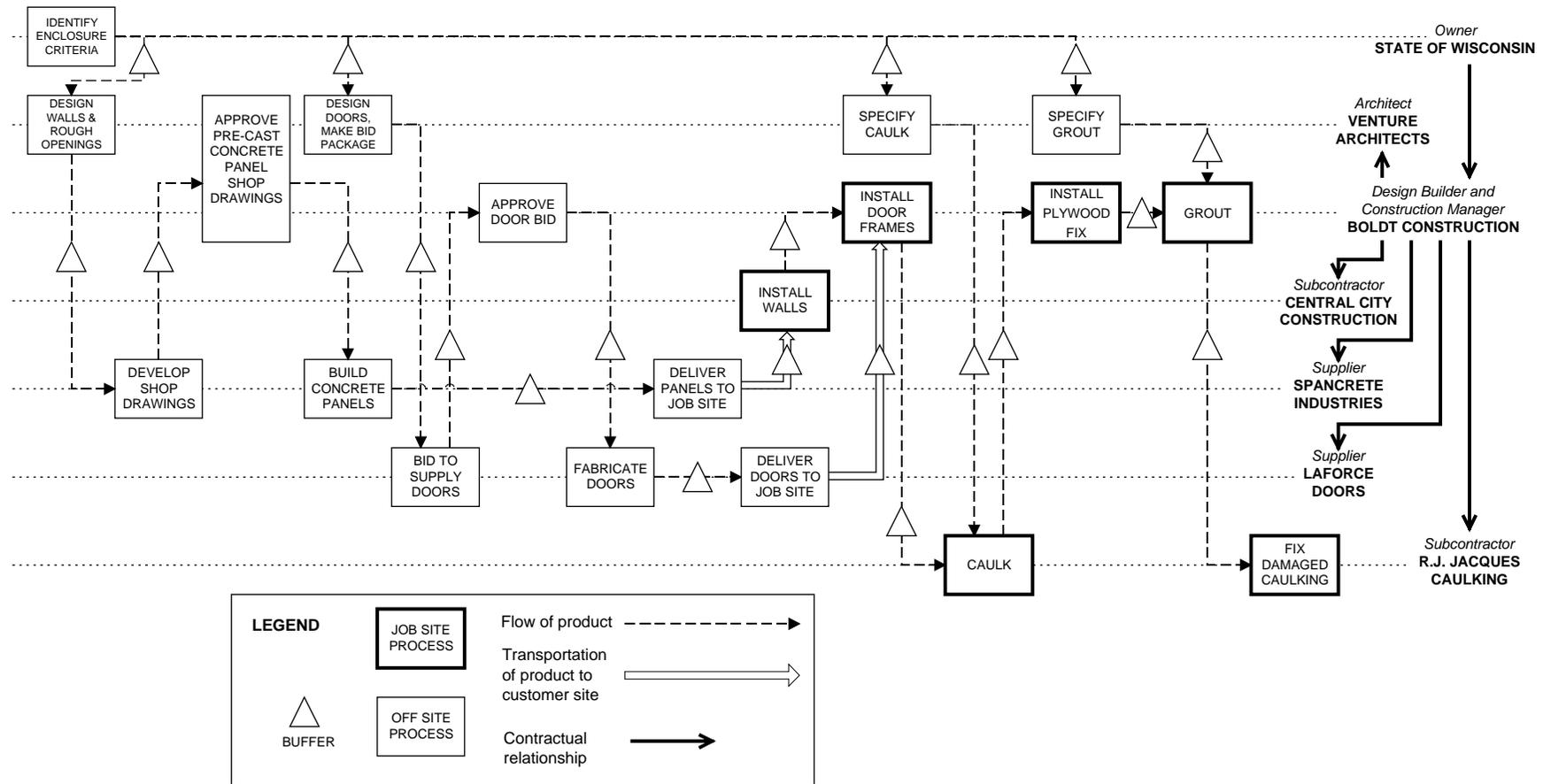
Figure 1: Supply and Contractual Relationships on Redgranite Correctional Institution
